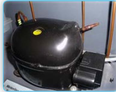
Process tube (crimped end)
