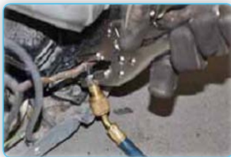
Piercing pliers connected to refrigerant line
