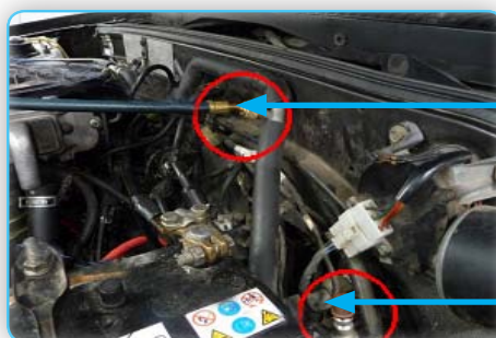
Vehicle air conditioner access ports
