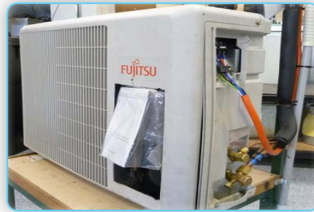
Split-system air-conditioner (external unit)
