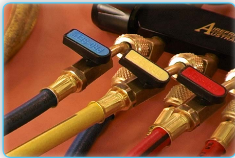
Service gauge manifold and service hoses with ball valves closed (left) and without ball valves (right)
