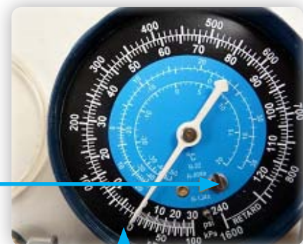
Align needle to zero mark
