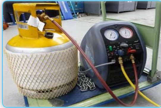
Recovery equipment set up on hand trolley
